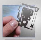
The mono-metal tuning fork sensor provides unrivaled stability with an extremely small margin of error. In this tiny device, experience sensitivity 50 times greater than that of any load cell.
