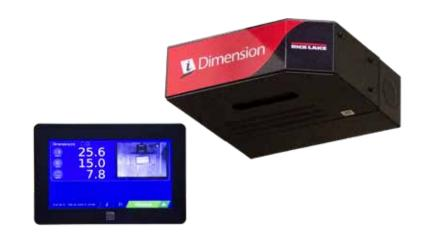
The iDimension Plus XL is specifically designed for integrators to provide flexibility in the installation of a dimensioning solution anywhere over a conveyor, table or scale from a pole, ceiling mount or support beam. Optional stand is available for ease of integration over a static roller conveyor at 60.2 inches (NTEP approved) or 79 inches above the platform.
