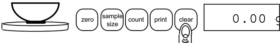
6. Remove the pieces from the container and press the **clear** key to return the scale to the weight display.
