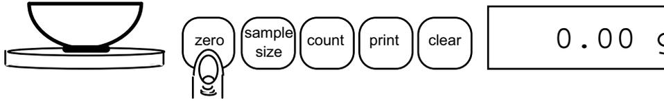
1. Place an empty container on the scale. Press the **zero** key.
