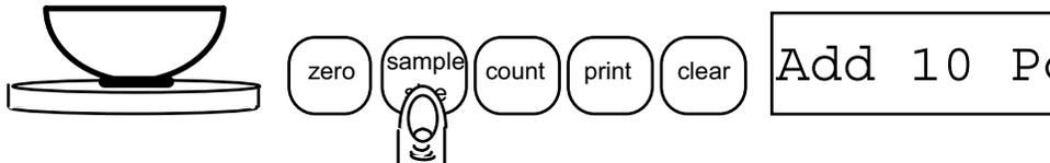
2. Press the **sample size** key. Each time the key is pressed the requested sample size will increase (i.e., Add 10, 25, 50, 100 PCs).
