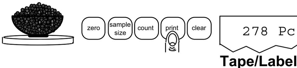
5. Press the **print** key to generate a tape/label or to transmit the data from the RS-232 port.
