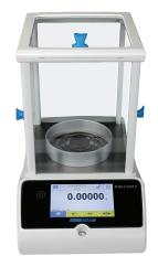
Semi-Micro Balances Dual-range models with 120g and 220g capacity and 0.01mg/0.1mg readability
